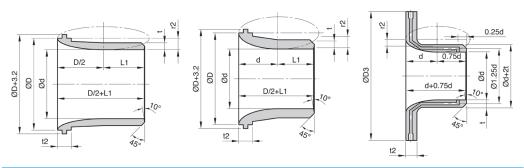
$0.5 \le \beta \le 0.8$   $L1 \le 0.6d \text{ or } \le D/3$  r2 = (D-d))/2  $2t \le D-(d+6mm)$   $3mm \le t2 \le 0.15D$ [A] High  $\beta$  Nozzle  $0.2 \le \beta < 0.5$   $0.6d \le L1 \le 0.75d$   $0.63d \le r2 \le 0.67d$   $3mm \le t \le 12mm$   $3mm \le t2 \le 0.15D$ [B] Low  $\beta$  Nozzle  $0.25 \le \beta < 0.5$   $0.63d \le r2 \le 0.67d$  t = 0.25d t2 = 38mm[C] Low  $\beta$  Nozzle, with Throat Tap
