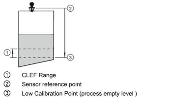
In applications with low dK materials we recommend setting CLEF Range to 0.5 m (1.64 ft) and **Position Detect (2.8.4.2.)** to Hybrid.
