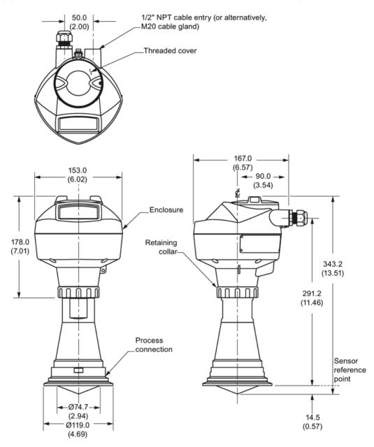
12.10 Hygienic encapsulated antenna (DN50 nozzle/slotted nut to DIN 11851)
