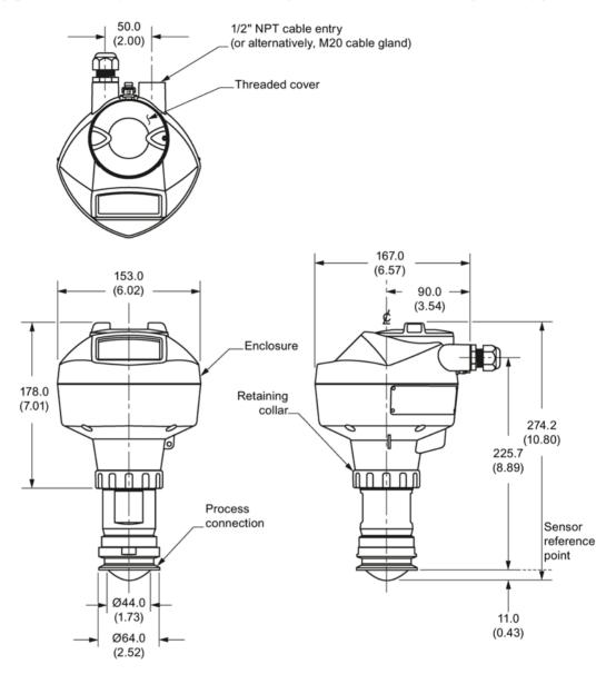
12.8 Hygienic encapsulated antenna (3" ISO 2852 sanitary clamp)
