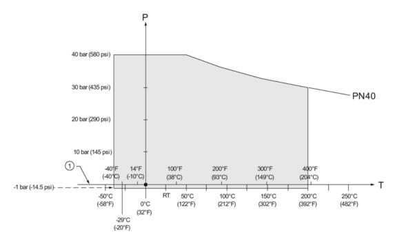
EN1092-1, PN40: DN50, DN80, DN100, and DN150
