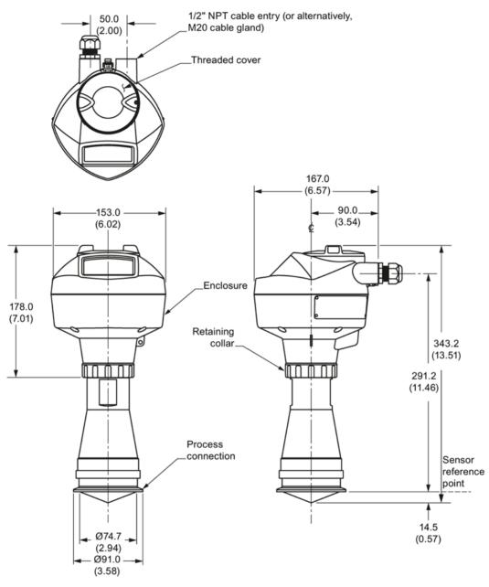
12.9 Hygienic encapsulated antenna (4" ISO 2852 sanitary clamp)
