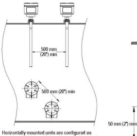
Horizontally mounted units are configured as point level switches. Mount diagonally if vertical space is restricted.
