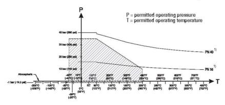
The curve denotes the minimum allowable flange class for the shaded area below.
