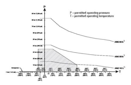
The curve denotes the minimum allowable flange class for the shaded area below.
