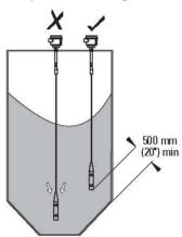
Note: Buildup of material or condensation in active shield area does not affect operation.
